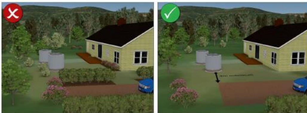
Figure 9: A good and a bad example of landscaping around a water tank and relation to hardstand areas (WAPC, 2021).
