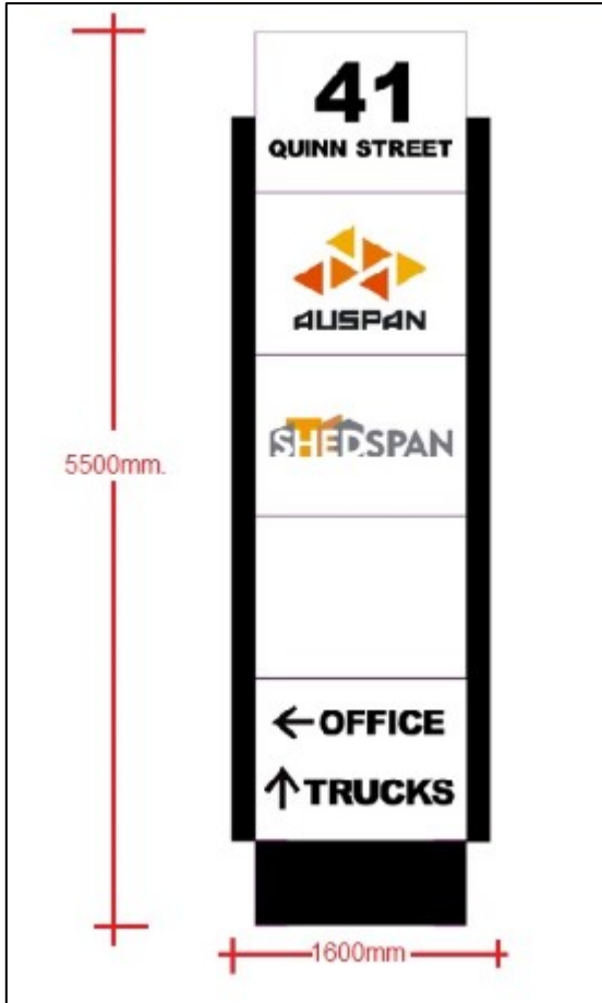
Large Pylon Sign at Office Car Park
